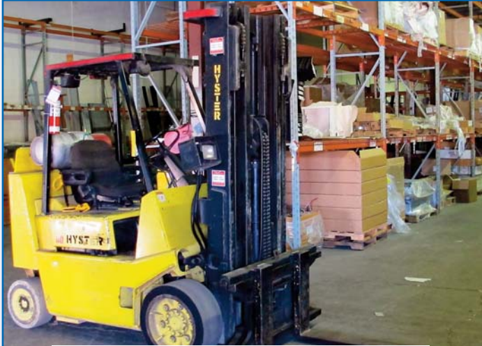
HYSTER S80XLBCS PROPANE FORKLIFT, 6,850LB CAP., 199.8" MAX LIFT, 3 STAGE, SIDE SHIFT, S/N D004D09343X
